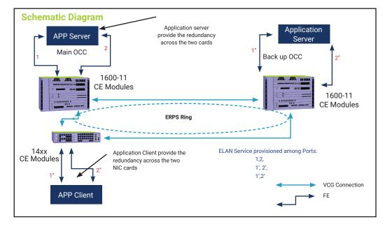
Advanced Protection Mechanisms: TJ1600 supports advanced traffic protection features to handle multiple fiber cuts in the network.
