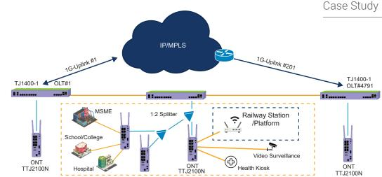
**Power savings:** TJ2100N can be solar powered and is available for installation in railway stations with erratic power supply in easily portable, ruggedized enclosures with batteries, solar panels and charging units. TJ2100N ONT supports Reverse PoE (RPoE) for corridor/basement installations (Ports 1 to 4), where power points could be scarce. Using RPoE, ONTs can be powered from Subscriber power supply.
