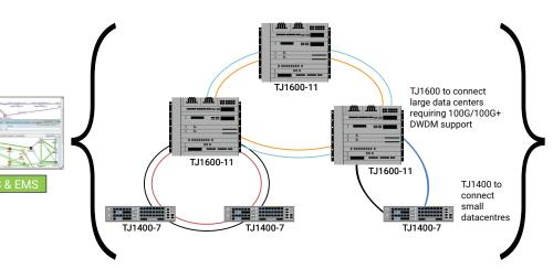
in-class density and feature set. TJ1600 can cost-effectively connect large data centers requiring 100G DWDM support. It enables extensive reuse of chassis commons, service cards, traffic slots, and interfaces during network upgrades or modernization.
